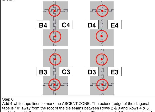
and in line with the center column seam, as shown. The other end of the tape is placed such that it is to the furthest corner of the tile but fully contained to one tile, as shown.
