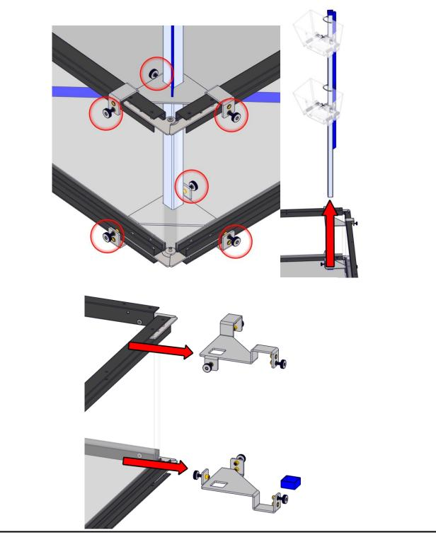
Step 2 Remove the Wing Nuts holding the Submersible to the tile and remove the Submersible assembly from the field.
