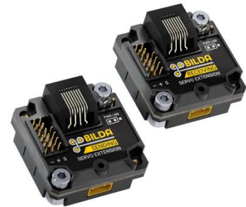
goBILDA 4-Channel Servo Extension via CAT6 (ILLEGAL)
