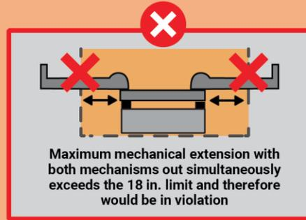
At maximum extension, a ROBOT in compliance will not exceed the maximum allowable vertical extension of 38 in. (96.50 cm) in one direction while maintaining the horizontal expansion requirements of 18 in. (45.70 cm) length and width perpendicular to the vertical height.
