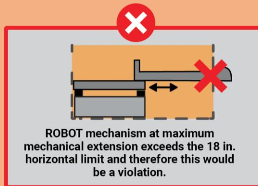
A ROBOT with a single mechanism that can extend out of both sides of a ROBOT would be allowed as long as the overall horizontal dimension at maximum mechanical extension does not exceed 18 in.
