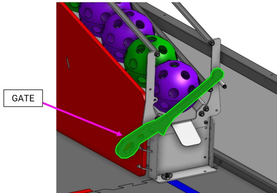
The GATE is a ROBOT-activated, push to open mechanism which will release ARTIFACTS which are CLASSIFIED on the RAMP (Figure 9-16).
