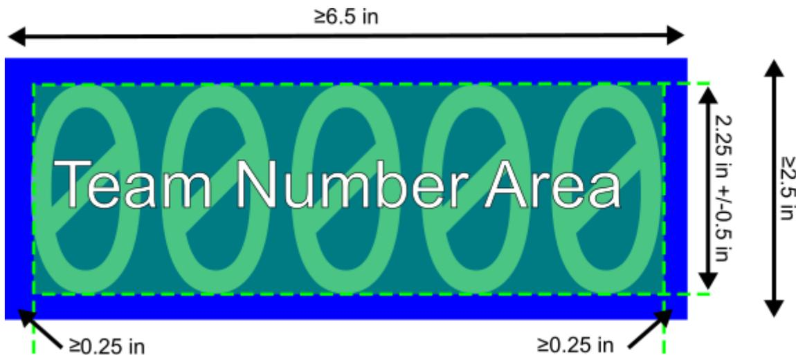
**R402 \*ROBOT SIGNS indicate your ALLIANCE.** Each ROBOT SIGN must contain a rectangle with a solid red or blue opaque background at least 6.5 in. by 2.5 in. (16.50 cm by 6.35 cm) in size to indicate their ALLIANCE color (Figure 12-3), as assigned in the MATCH schedule at the event. Visible markings on ROBOT SIGNS when installed on the ROBOT, other than the following, are prohibited:
