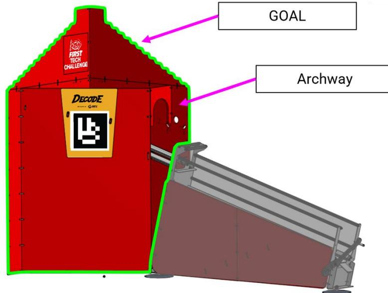
The opening of the GOAL is approximately 26.5 in. (67.30 cm) wide and 18.3 in. (46.45 cm) deep. The top lip of the GOAL is 38.75 in. (98.45 cm) from the surface of the TILE. The maximum height of the backboard with the FIRST Tech Challenge logo is 15 in. (38.10 cm) from the open top of the GOAL (Figure 9-9).
