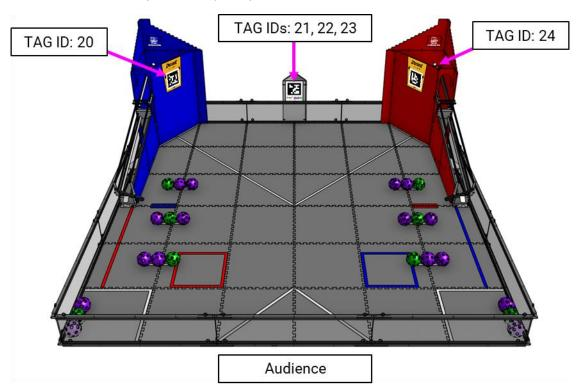
Figure 9-18: AprilTag Locations on the DECODE FIELD
