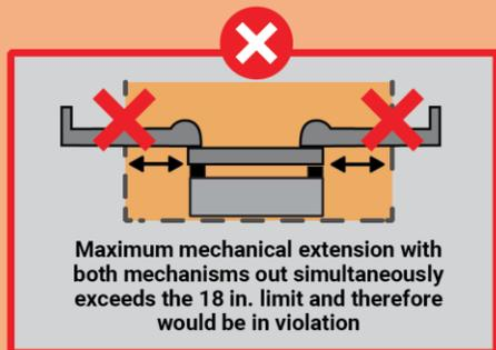
Maximum mechanical extension with both mechanisms out simultaneously exceeds the 18 in. limit and therefore would be in violation
