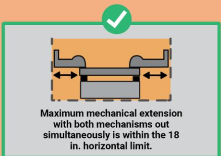
Maximum mechanical extension with both mechanisms out simultaneously is within the 18 in. horizontal limit.
