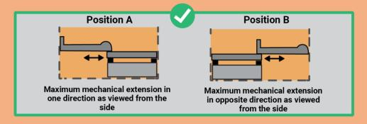
A ROBOT with multiple mechanisms that are not mechanically linked that can extend out of both sides of a ROBOT simultaneously would NOT be allowed if the overall horizontal dimension at maximum mechanical extension exceeds the 18 in. limit.
