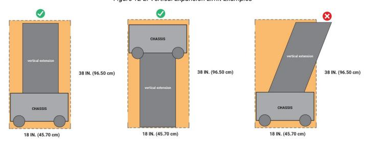
Any extension beyond the maximum expansion limit during ROBOT operation is considered a violation of this rule. This includes flexible extensions (e.g., surgical
