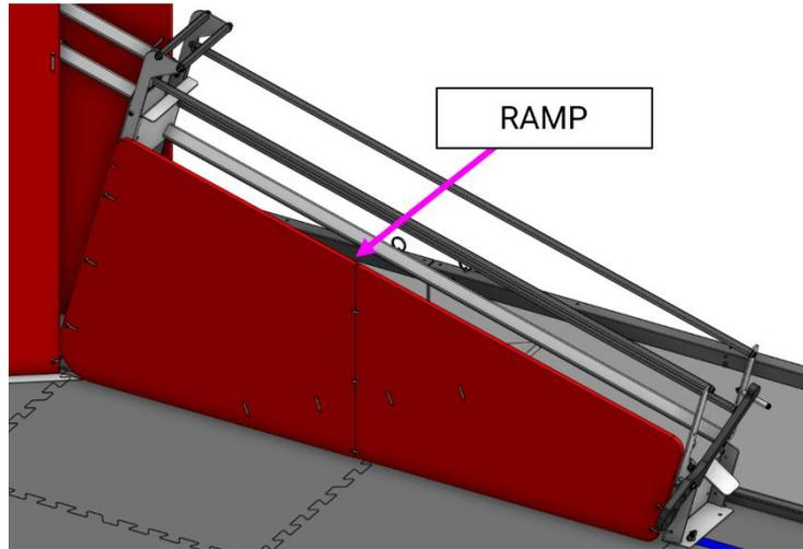
In most cases exactly 9 ARTIFACTS will fit on the RAMP as CLASSIFIED before newly entered ARTIFACTS will OVERFLOW, but sometimes ARTIFACTS LAUNCHED into the GOAL at a high velocity or with significant spin may skip over the 9<sup>th</sup> open CLASSIFIER slot and count as OVERFLOW. This is a normal FIELD operation and not an ARENA FAULT.
