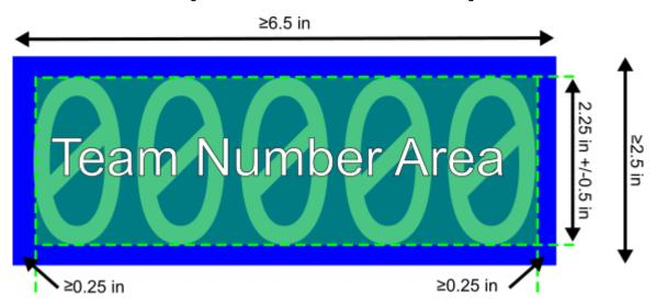
Figure 12-3: Team Number ROBOT SIGN Sizing
