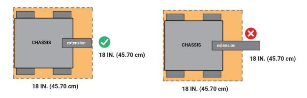
Figure 12-2: Vertical Expansion Limit Examples
