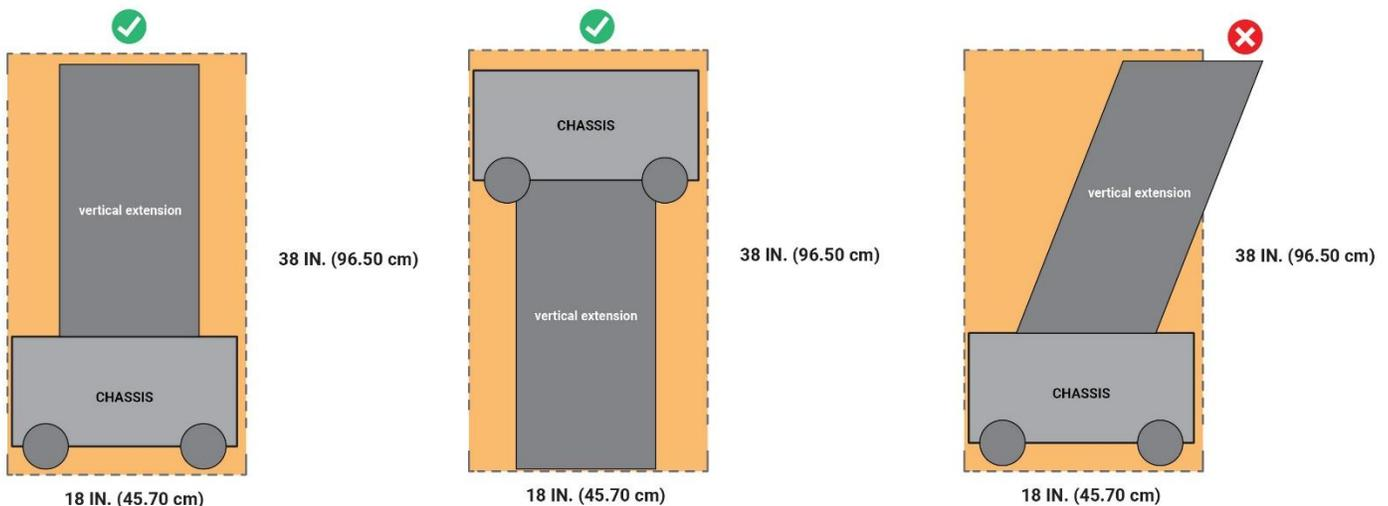
Any extension beyond the maximum expansion limit during ROBOT operation is considered a violation of this rule. This includes flexible extensions (e.g., surgical
