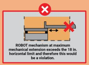
A ROBOT with a single mechanism that can extend out of both sides of a ROBOT would be allowed as long as the overall horizontal dimension at maximum mechanical extension does not exceed 18 in.
