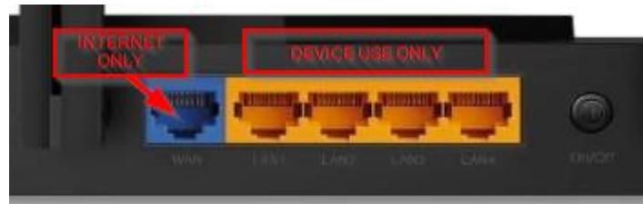
Figure 2: WAN (blue) and LAN (yellow) ports on a Wi-Fi router.
