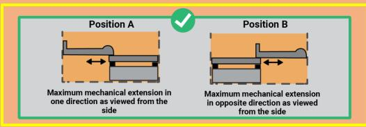
A ROBOT with multiple mechanisms that are not mechanically linked that can extend out of both sides of a ROBOT simultaneously would NOT be allowed if the overall horizontal dimension at maximum mechanical extension exceeds the 18 in. limit.
