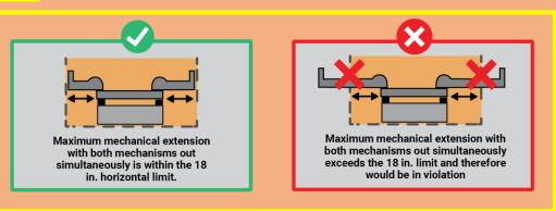
At maximum extension, a ROBOT in compliance will not exceed the maximum allowable vertical extension of 38 in. (96.50 cm) in one direction while maintaining the horizontal expansion requirements of 18 in. (45.70 cm) length and width perpendicular to the vertical height.
