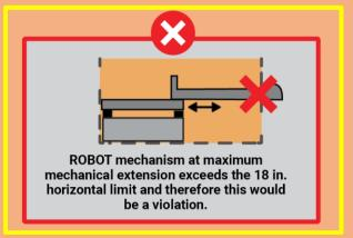
A ROBOT with a single mechanism that can extend out of both sides of a ROBOT would be allowed as long as the overall horizontal dimension at maximum mechanical extension does not exceed 18 in.
