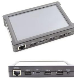
Figure 4 - Expansion Hub or Control Hub configured with REV Driver Hub (shown)
