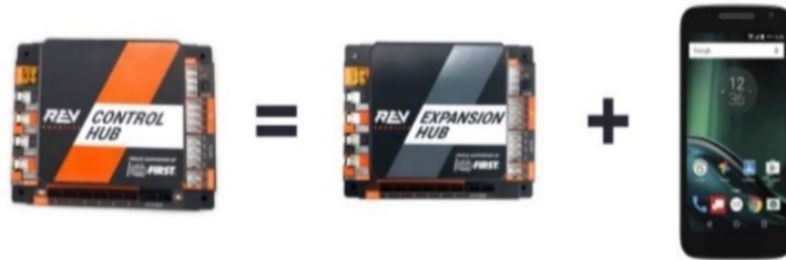
Figure 3 - A Control Hub is a Robot Controller with an internal Android device
