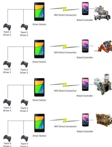
Figure 2 - Each Team will have its own DS, RC and wireless network connection
