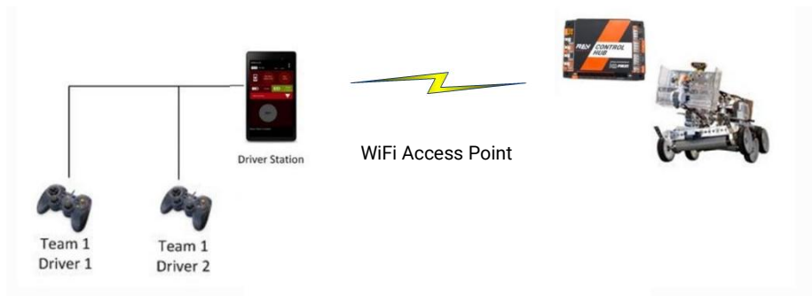
Figure 1 - Each DS-RC pair has its own unique wireless connection
