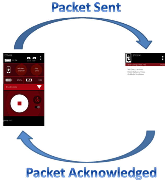
Figure 30 - Ping time represents the time it takes for a packet to be sent to and acknowledged by the Robot Controller.
